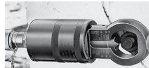
Align mark on cutter blade with scale.
